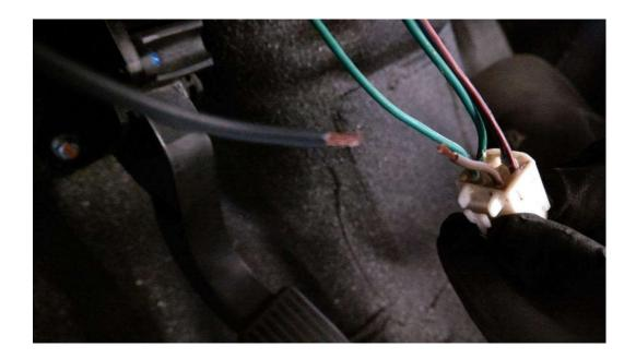
Connect the grey with black striped wire to the factory brown wire at the plug end of the brake switch as shown with supplied butt connector.
