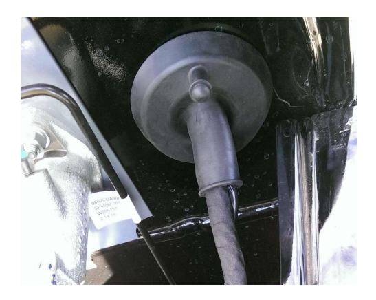
Split the remaining harness branches near the large factory harness plug on left fender. Route the single grey wire under the brake master cylinder along the factory harness and to the frame rail ending at the left rear of the vehicle securing it to the existing wires as you go along with zip ties.
