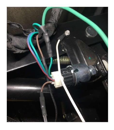
Secure the flasher and connecting wires under the dash with zip ties.
