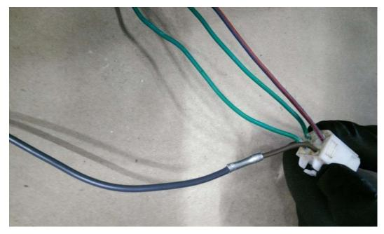
Connect the black wire to the remaining end of the factory brown wire.
