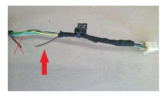
Attach the single grey wire to the cut brown wire closest to tail light plug and terminate the remaining wire. Secure any loose wires to existing wire harness.
