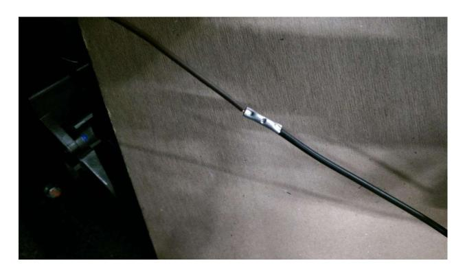
Cut one of the green wires (doesn't matter which one) approximately  $1\frac{1}{2}$ " from the plug and splice in supplied green wire with stepped butt connector as shown.
