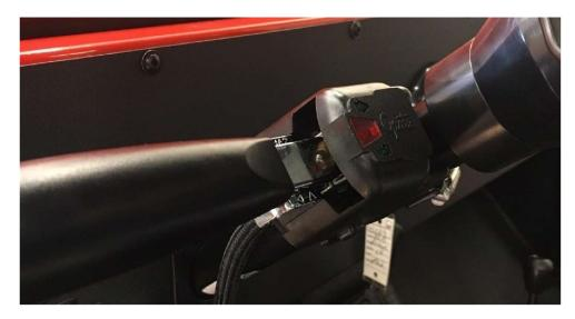
Mark and drill a 34" hole into the plastic panel below the steering column as shown.
