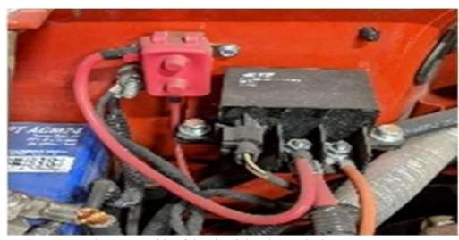
6) Connect the "BAT" side of the circuit breaker to the battery
