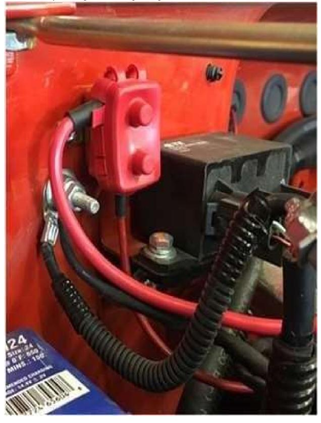
3) Splice the thin red wire from the fuse panel into the pink with yellow tracer wire from the unused connector on the backside of the dash panel labeled "Side/Rear LED Light" this is a keyed 12V power source used to trigger the auxiliary fuse panel relay.
