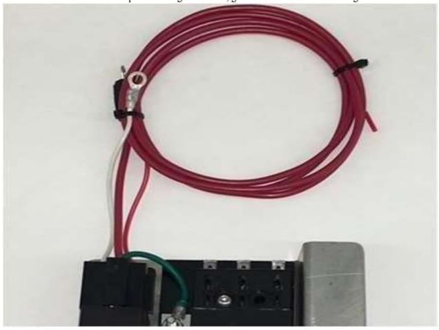
5) The large red wire from the fuse panel gets connected to the "AUX" terminal of the circuit breaker.
