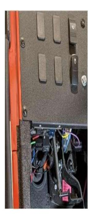
2) Mount the included circuit breaker to the firewall above the battery. Be cautious of any wiring on the inside of the firewall that may be damaged when drilling or using sheet metal screws.
