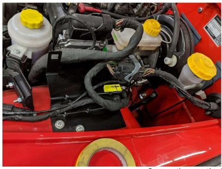
Drill a ¼" hole into the bracket located on the driver side fender as pictured
