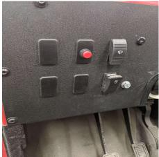
Ground the black wire to an adequate ground and attach one terminal of the switch to a fused 12v source and attach the other terminal of the switch to the positive terminal of the pump.
