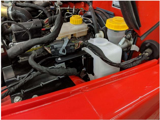
Fill the reservoir with proper washer fluid and test. It may be necessary to operate the pump 4 to 5 times to prime. You will also need to aim your nozzles to spray in the desired location on the windshield (using a small sewing needle works best).
