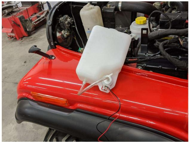
Attach the long hose to the reservoir output and zip tie along the brake booster hose and run it through the firewall and attach it to the t-fitting under the dash that connect your washer nozzles
