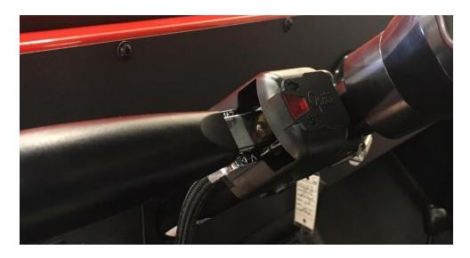
Mark and drill a ¾" hole into the plastic panel below the steering column as shown.
