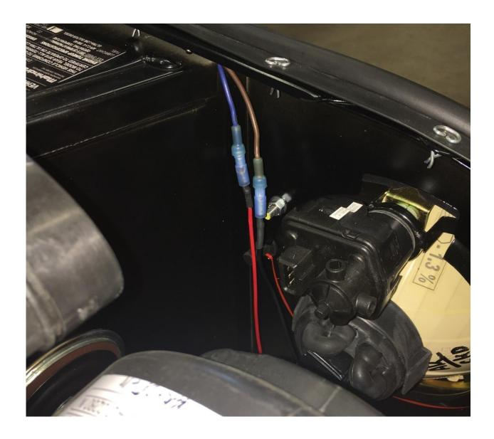
Verify that all connections are heat shrunk, correct, and that no wires are routed in an area where they may be damaged or crushed.
