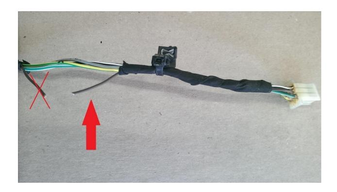
Attach the single yellow wire to the cut brown wire closest to tail light plug and terminate the remaining wire. Secure any loose wires to existing wire harness.
