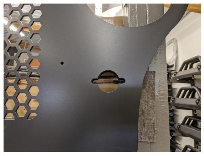
Next, measure from the center of your mark 1 3/32" on either side and drill Two 3/16" holes for the signal light mounting bolts through both the plastic cover and the steel structure behind as shown. Drill a  $1\frac{1}{2}$ " hole at the center mark for the marker light. Refer to the template included with the kit. If using our Roxor grille, use it as a template, and drill through only the steel structure.
