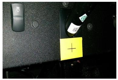
Carefully feed the wiring harness through the drilled hole and clip the grommet into place. **Important:** Avoid routing wires against the pedal return springs.
