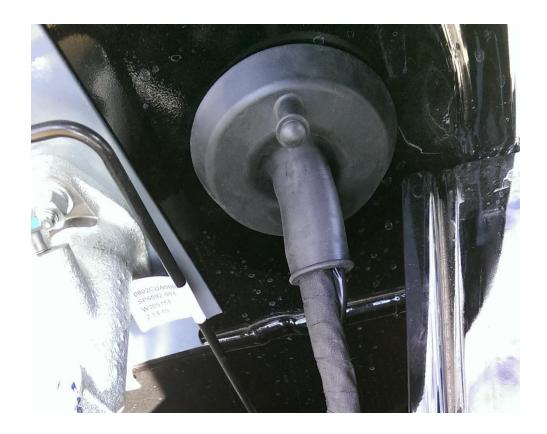
Split the remaining harness branches near the large factory harness plug on left fender. Route the single yellow wire under the brake master cylinder along the factory harness and to the frame rail ending at the left rear of the vehicle securing it to the existing wires as you go along with zip ties.
