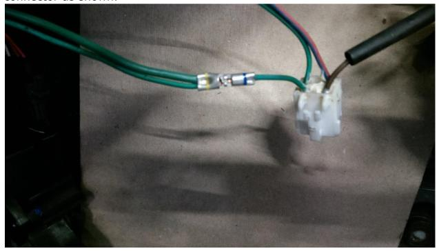
Connect the green, blue and yellow wires to the supplied flasher as follows: Green=X Blue=P Yellow=L
