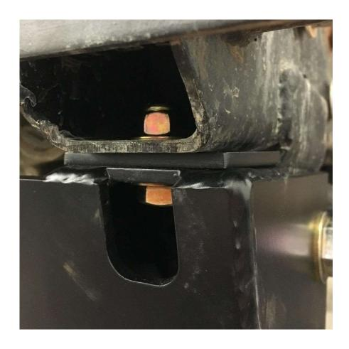
• If the shackle mount is welded in the most common area, and not lower than standard, you will not need this spacer. Shown.
