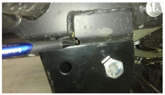
Also reuse the original Mahindra rear spring bolt (with grease zerk) onto the front of the spring to the OTR Cross Member. (Torque to 94 Ft. Lbs.)
