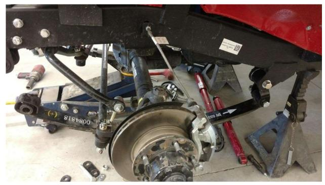
• Remove the Mahindra front shackle bushing, located on the front of the frame rail.
