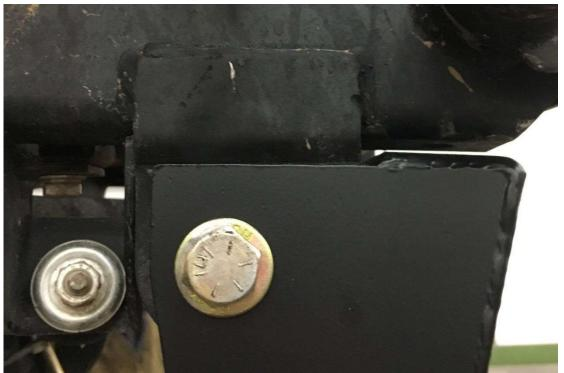
• If this is the case, you will need to install our included spacer with the 7/16" bolt between the cross member and frame. As shown in the following picture.
