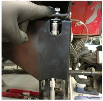
• Due to Mahindra's manufacturing tolerances, you may also need to die grind the original shackle mount.
