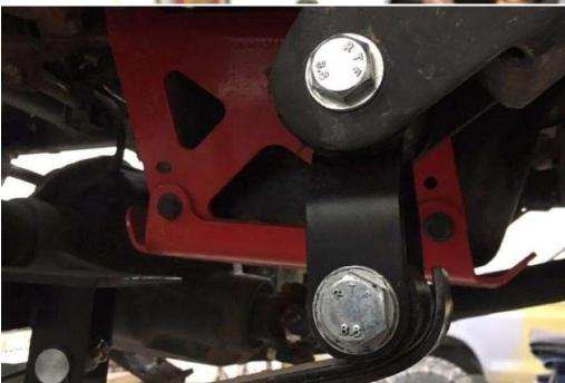
shackle utilizing the existing Mahindra spring bolt. SNUG BOLT Wait to torque bolts until the vehicle weight is back on suspension. (Torque to 93 Ft. Lbs. with the weight of the vehicle on the suspension.)
