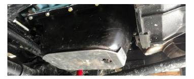
4. Once installed and dried, you may take an RTV type sealant and make a bead sealing out debris from between the skid plate and oil pan.
