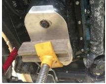
3. Next, stick the skid plate to the bottom of the oil pan, and then use a jack to apply pressure and let set up for at least one hour.
