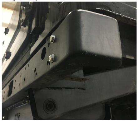
• Locate the 12mm-1.75 metric thread tap from the hardware. Use the thread tap to tap the bottom two center holes. A 7mm open end wrench fits on the tap. (Only required on 2018-2019)
