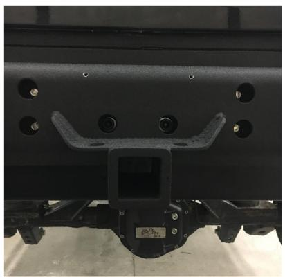
Locate the remaining (4) 8mm flange head bolts and steel lock nuts. Install these into the two outer sets of holes.
