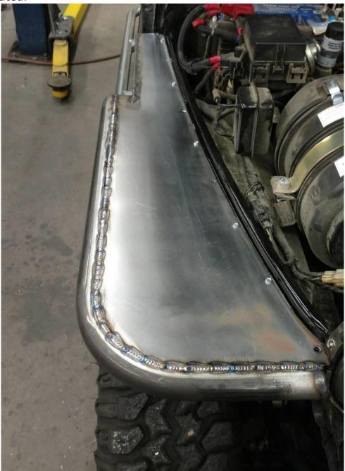
• When you are reinstalling the fenders, use the supplied ¼" bolts and nuts to reinstall. You will need to use the fenders as a guiding template to drill mounting holes into the existing original fender material to install. Remount the factory hood hold downs.
