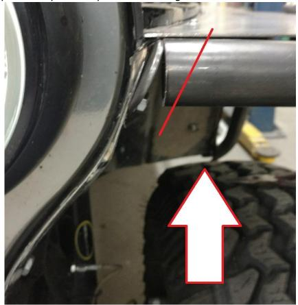
Trim the tubing to fit onto the tab as shown below, while fitting and lining up the tube with the rest of the top plate. Once fit-up, tack the tubing in place
