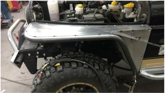
• Once you have each side fit-up and tack welded, you can remove them for final welding and metal finishing. If a weld is not desired on the top visible side of the fender, you can tack together and stich weld the inside of the tubing and plates together. Seam seal the top side.
