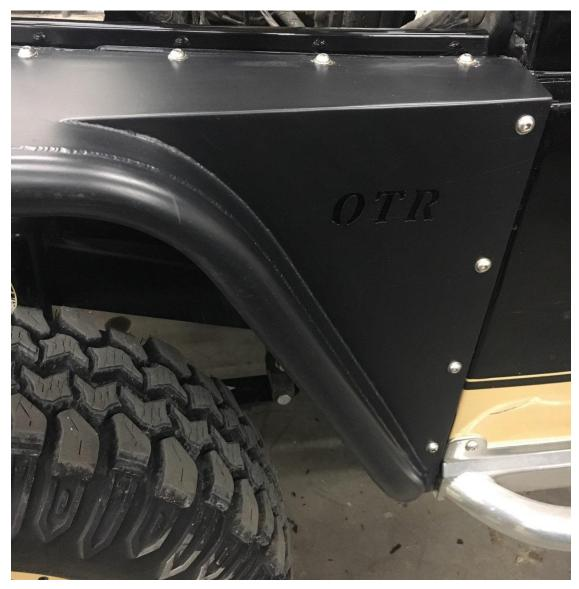
The tube fenders will not sit flush with the body. If you want to adjust them flush, you will need to notch the 4 OE fender mounting holes located inside the fender, perpendicular to the 4 tube fender bolts along the back edge. The top 2 bolt holes will be notched on a diagonal "up and out" on the fender. The bottom 2 bolt holes will be notched on a diagonal "in and down" on the body.
