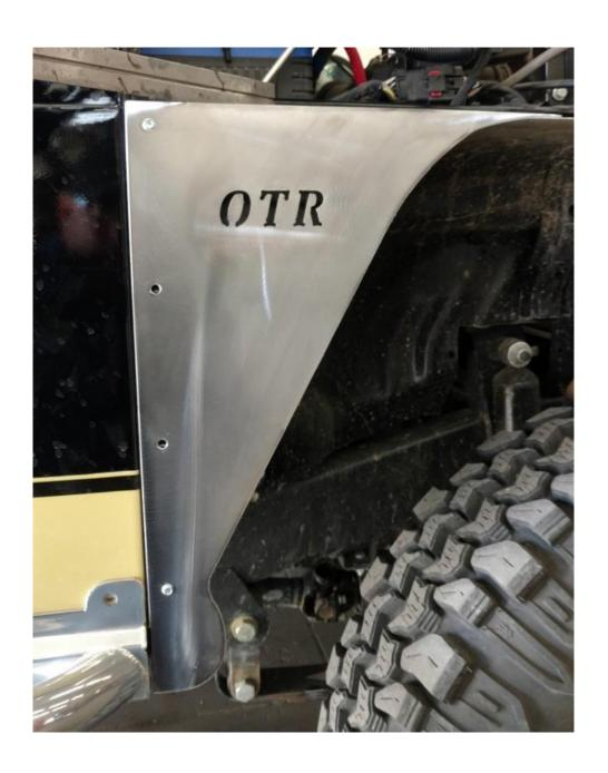
Fit the top piece with some temporary zip screws. You will need to drill ¼" holes for the mounting bolts after you have fit and welded everything up.
