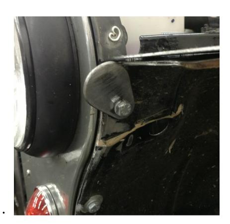
• Clamp the tubing to the fender by the footwell area, so that it is loosely in place as you fit-up the mounting tab.
