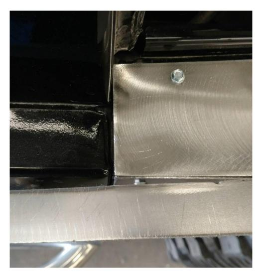
You can begin to tack the top plate to the bottom plate once they are fit up and in the correct position. (If you do not want a weld to be visible on the top, tack weld the plates together on the inside.)
