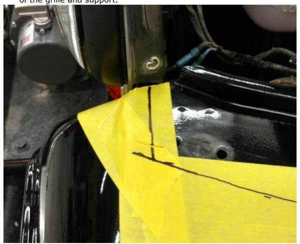
You may drill a couple of holes to cut between with a body saw along the fender lines.
