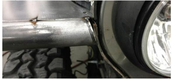
Start forming the rear piece of the top plate to the rear of the tubing, and down to the bottom of the side plate. Tack this piece in place as you fit-up and form it to the arch of the tube.
