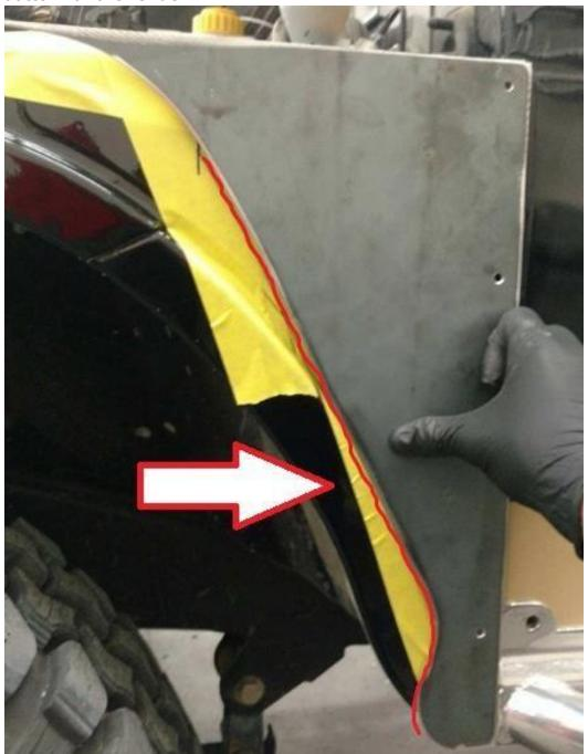
Following the top flange on the fender, measure and mark a series of lines 3" outward from the flanges and connect the lines.
