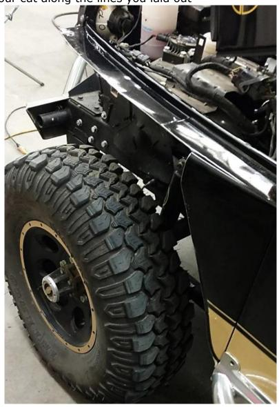
• Trim the remaining part of the fender that hangs out past the grille. Stay just on the outside of the factory seam towards the front.
