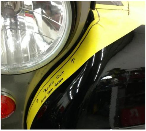
Mark the top of the fender roughly as shown below close to the center of the grille and support.
