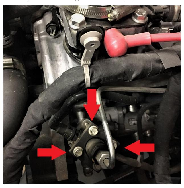
• Then, locate the supplied intake hold down, and ¼" bolt.
