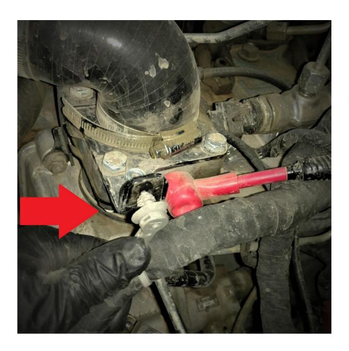
• Next, remove the three upper bolts on the lift pump.
