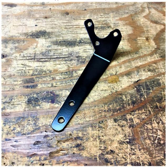
• Using the factory three lift pump bolts install the intake hold down. Torque to the manufacturer recommended specs. Use the supplied ¼" nut and bolt to fasten the hold down to the intake where the wiring harness was fastened.
