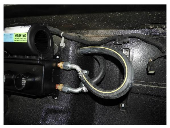
• Run each end of the supplied heater hose through the grommets into the firewall. Slide the hose onto the 45-degree fittings and secure them with hose clamps as shown in the picture above.
