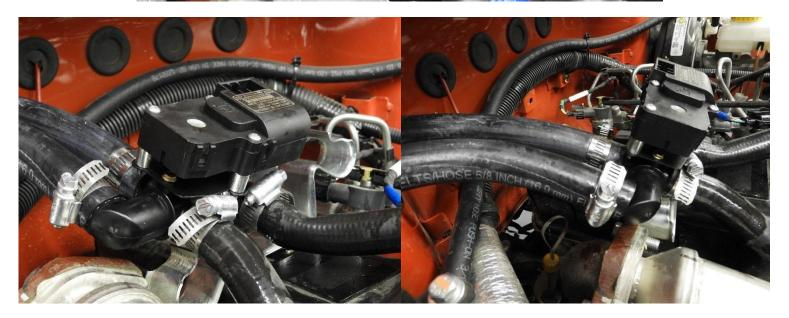
• If the EGR has been removed, splice into the hose that runs from the thermostat to the EGR cooler with our supplied hose barb and a strait section of heater hose running to the 4-way valve.
