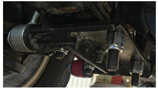
• Remove the front spring to shackle mounting bolt.
