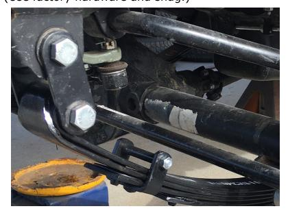
Now mount the rear of the spring pack into the rear spring mount with the factory bolt with the grease fitting. You may need to use a rubber mallet in order to get the leaf spring pack up into the rear spring mount. Clearance will be tight as intended. If needed you may file the steel bushing just enough to make a tight fit into the rear spring mount.
