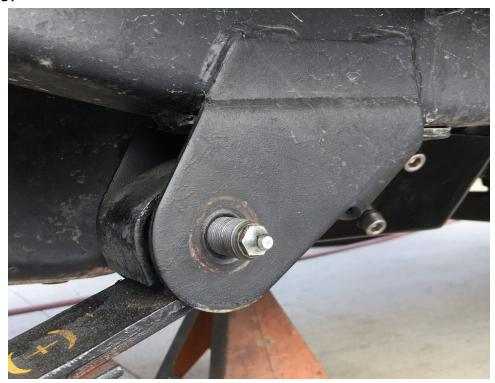
The factory spring is now removed. (You will reuse this factory spring mounting hardware.) • Locate new springs. The full wrapped end of the spring pack goes towards the rear of the vehicle.
