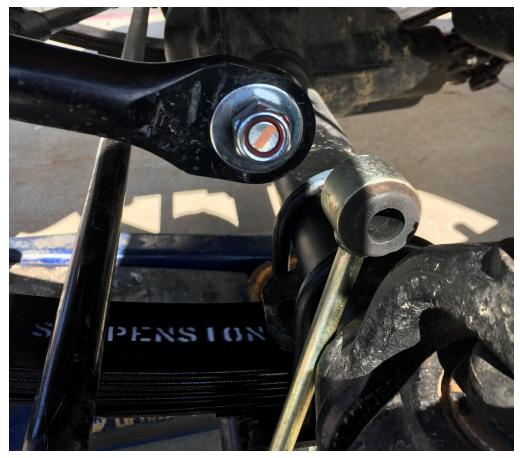
• Remove U bolts, along with the factory spring mounting plate.
