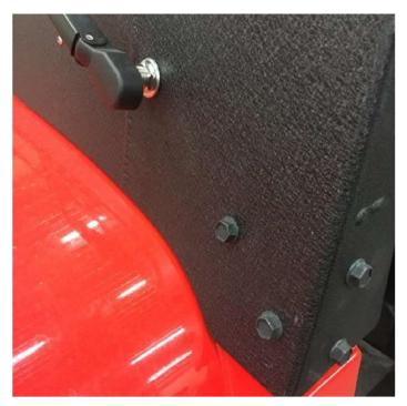
Install the supplied quick release clamps on the windshield frame as shown. (Leave the hardware loose until it is clamped to roll bar, adjust to fit then tighten hardware)
