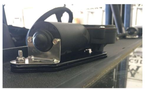
Make sure to keep wiper motor wiring harness out of the way of the hinge closing and opening.
