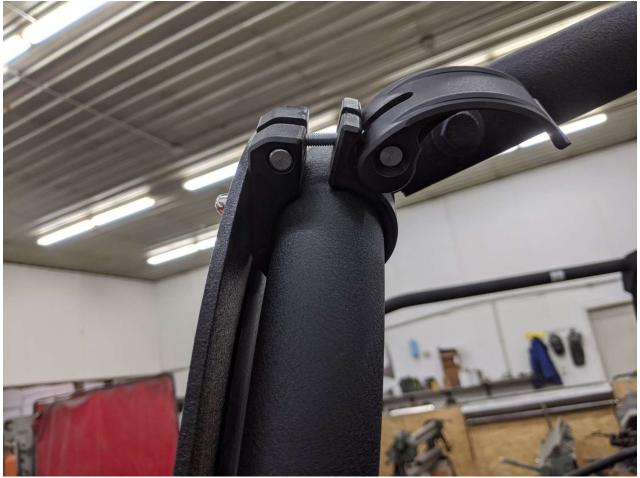
Take the supplied 5/16-inch stainless bolts and fender washers and mount them through the bottom center holes in the windshield frame that line up with the factory Roxor holes in the cowl to better solidify the mount. Install them with the fender washer and nut inside and under the dash, and the button head on the outside of the frame.
