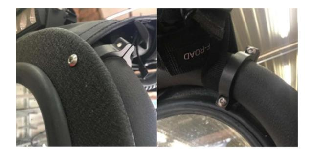
• Take the supplied 5/16-inch stainless bolts and fender washers and mount them through the bottom center holes in the windshield frame that line up with the factory Roxor holes in the cowl to better solidify the mount. Install them with the fender washer and nut inside and under the dash, and the button head on the outside of the frame.
