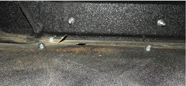
• Once all of the fasteners are loosely installed, you may go back through and tighten up all hardware.
