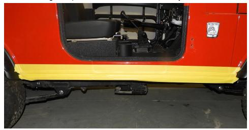
Take the Rox Sliders, and fit up to the side of the Roxor. You may use vise grips or other clamps to clamp them to the side in the mounting location, (mask off the area of the Rox Slider that the clamp is holding onto.) MAKE SURE TO ORIENTATE THEM THE CORRECT WAY- The square end faces forward, and the other end is cut at an angle to fit the rear fender line as shown below.
