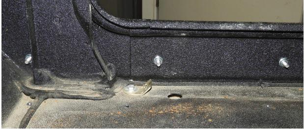
• Use the Flange Head Bolts, and remaining Serrated Flange Nuts to loosely mount the bottom of the Rox Sliders up into the bottom tub of the Roxor.
