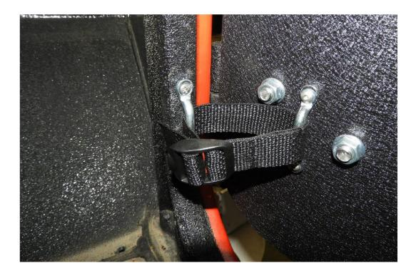
o If you are using the footman loops, align footman loop onto door frame in line with the door mounted footman loop. Using the supplied #8 screws, mount the footman loop in the center of the frame, as shown.
