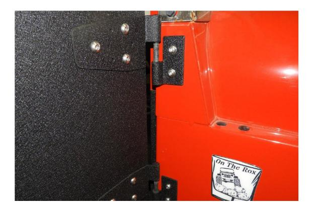
• Align the door gap by closing door and adjusting loosely fastened hinges to satisfaction then tighten the mounting bolts.
