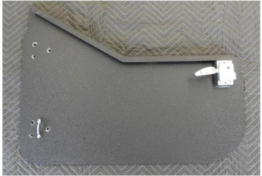
• Locate the door hinge sets. Match them up with the doors as shown in the picture below. Hinge studs will face outward and down. The hinges with the 3 smaller holes will be mounted to the top of the door. (Holes are for an optional mirror.)
